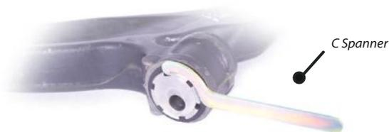
Figure 3 - Adjusting the Geometry
